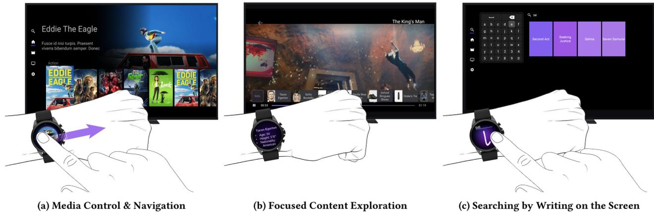
**Figure 1:** WristFlick is a smartwatch-based system designed for interacting with smart televisions. It allows users to browse channels, manage media playback, and view extra content like cast and soundtrack information using simple taps and flicks on the smartwatch. Users can also write directly on the smartwatch screen to search for specific channels or titles.
