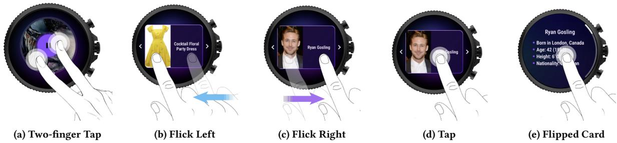
**Figure 9: Focused content exploration with WristFlick:** (a) demonstrates performing a two-finger tap to activate focused content mode; (b) and (c) demonstrate flicking left and right to view the previous and next item cards, respectively; (d) shows a tap to flip the card for more details; and (e) displays the flipped card with additional information.
