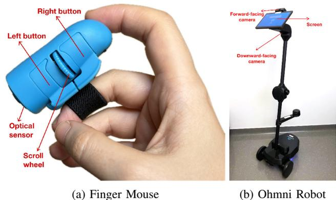
Fig. 3: The finger-wearable mouse and the telepresence robot (simulated in the study) used in this work.
