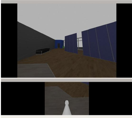
Fig. 4: The robot control graphical user interface (GUI) used with both methods. The top section displays the forward-facing camera view, while the bottom section displays the downward-facing camera view.
